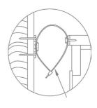
3. Move the furniture to it's final position and align the bracket on the furniture with the bracket on the wall. Thread the strap through the bracket as shown, and tighten until snug. Do not over-tighten.
